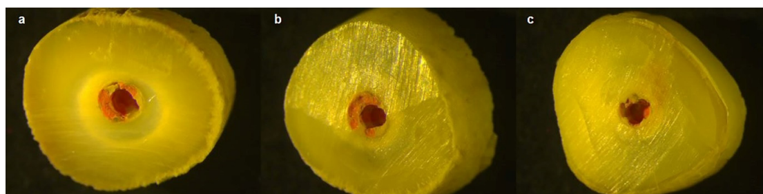
Figure 2. Stereo-microscope images of samples (a: A sample with mixed failure in the coronal section; b: A sample with mixed failure in the middle section; c: A sample with adhesive failure in the apical section).
