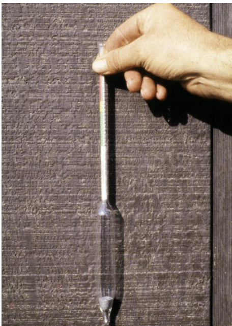
C-72: Colostrometer. A commercially available hygrometer for measurement of immunoglobulin concentration in colostrum. Commonly used for this purpose but there are limitations to its accuracy for this purpose.
