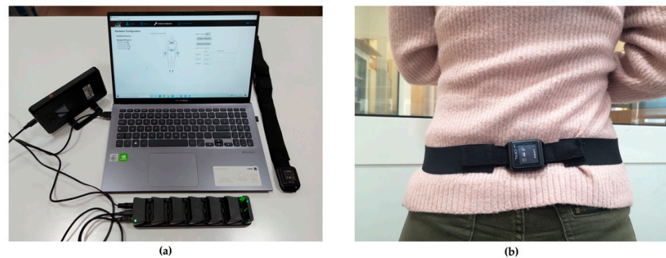
Figure 4. (a) Opal System; (b) Opal sensor positioning. Reproduced with permission from [34]; published by Multidisciplinary Digital Publishing Institute, 2021.
