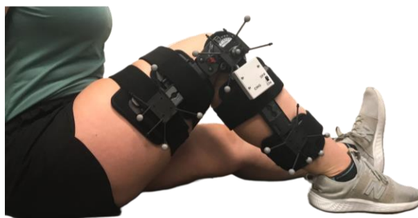
Figure 2. Instrumented knee brace with rigid body bases and reflective markers attached at the thigh, knee, and shank.
