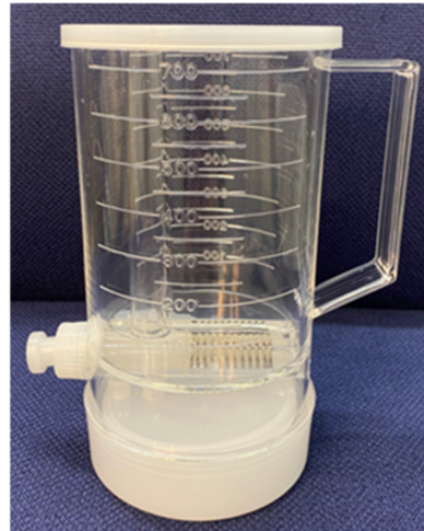
Figure 2. An aliquot cup that allows one-40th of urine samples to be collected personally at each time of voiding during 24-h urine sampling [39,43].
