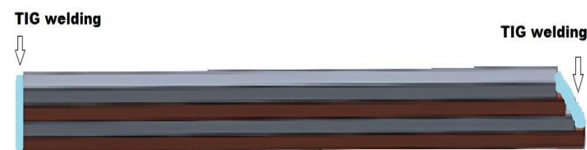
Figure 2. TIG welding with addition of aluminum at both ends of the initial sample.
