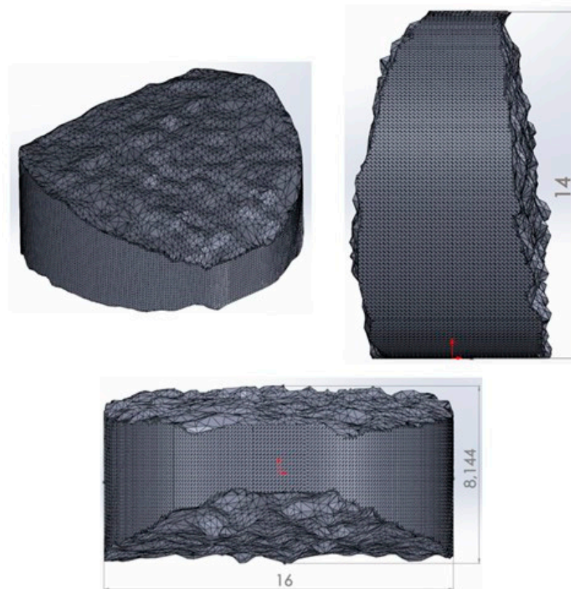
Figure 5. CAD model of the implant of the intervertebral disc (height, width, and thickness of the model).
