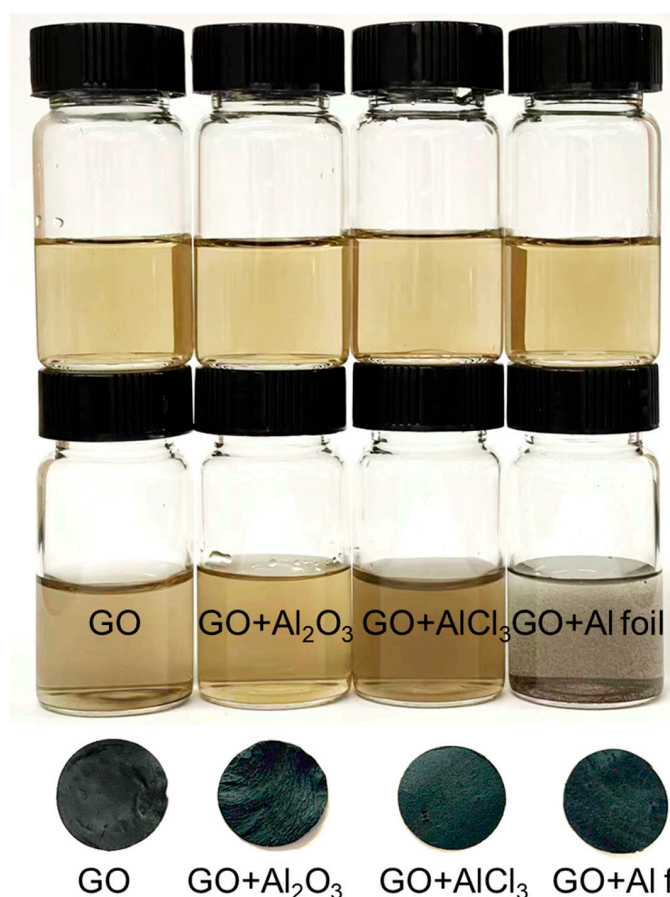
Figure 9. Comparison of the GO sheet solution (top) to sonicated solutions of the GO, AGO ( \text{Al}_2\text{O}_3 ), AGO ( \text{AlCl}_3 ) and AGO (Al foil) membranes (bottom).
