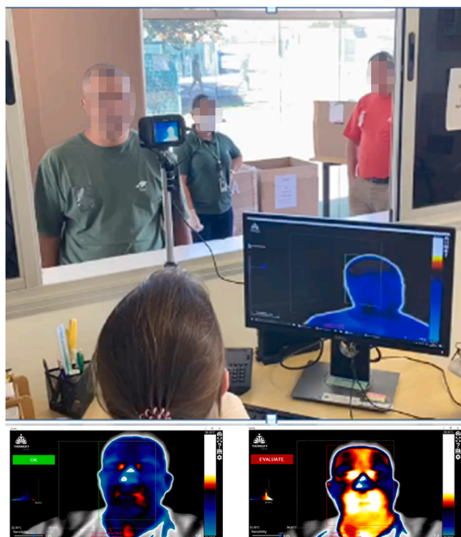
Fig. 3. Typical rapid infrared image sampling system that was set up in an external, non-thermally controlled environment at the entrance of all selected companies (top). At the bottom 2 examples of the utilized facial infrared images CNN algorithm results are shown either with a green OK (left image) to classify the individual in the no fever group or with a red EVALUATE (right image) to classify the individual in the fever or subfebrile group.
