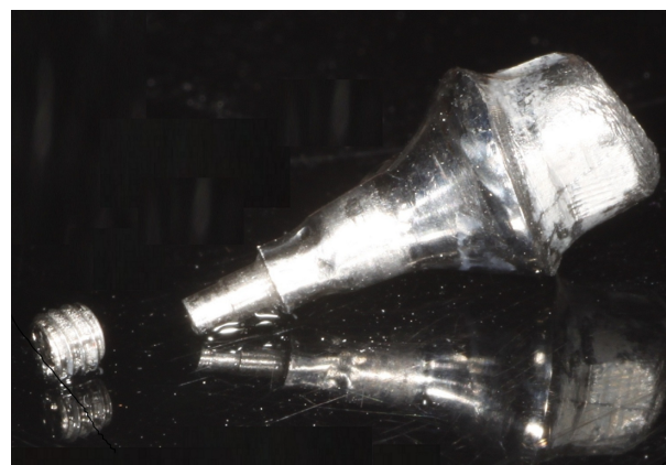
FIGURE 9 View of fracture only at the end of the central screw
