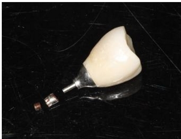
FIGURE 7 View of fracture both at the neck of abutment and at the screw
