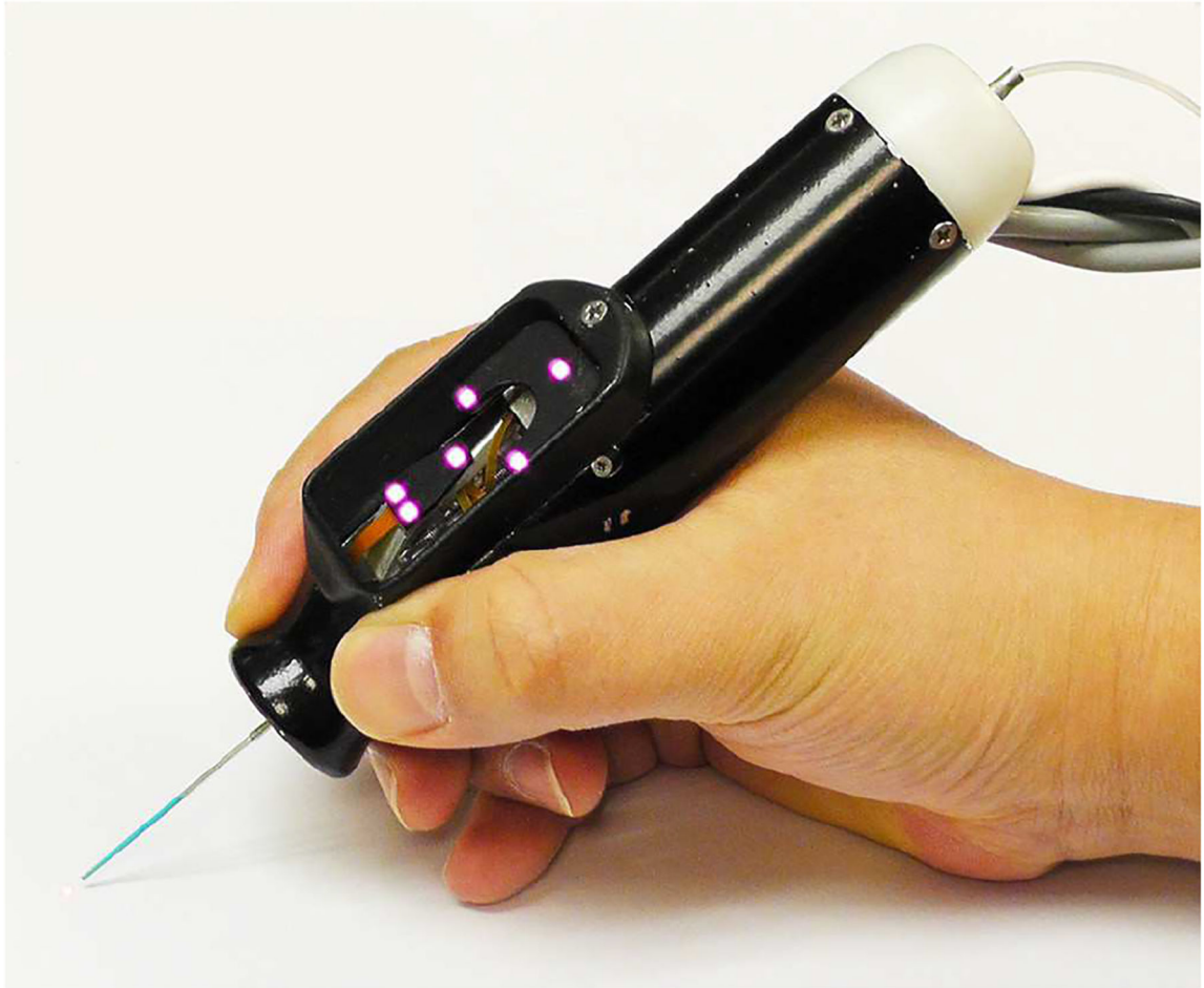
Fig. 6. The Micron: a handheld micromanipulator developed by Carnegie Mellon University. Image © Cameron Riviere.
