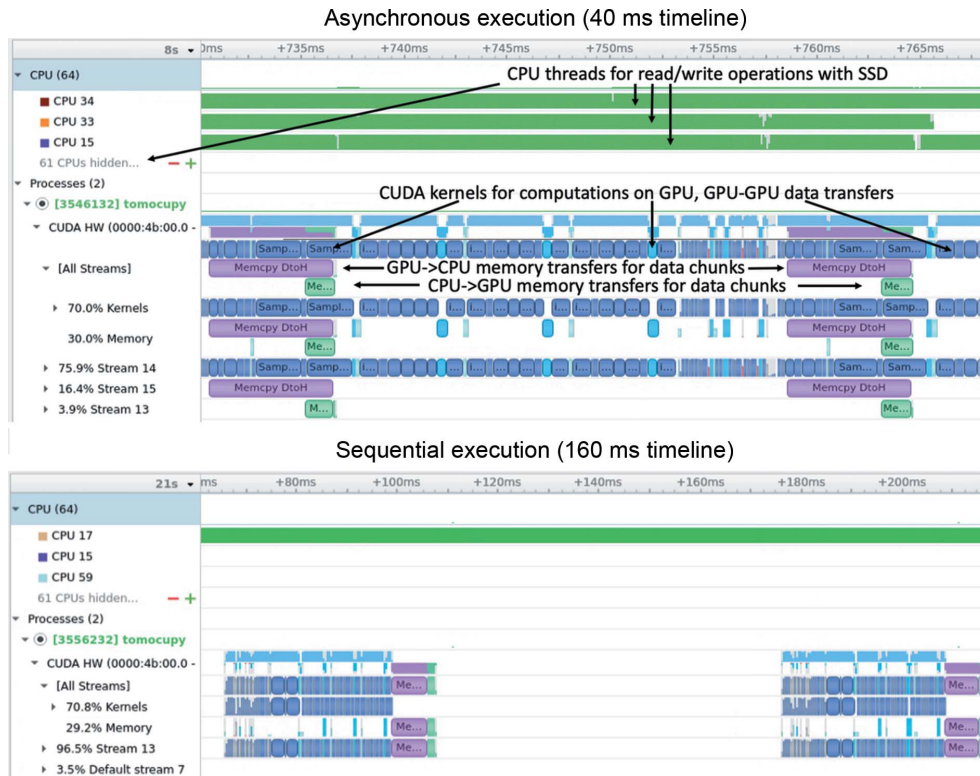
Figure 2 Timeline view report from the Nvidia Nsight System tool for asynchronous and sequential execution of reconstruction with TomocuPy . Reconstruction was performed for a 2048 \times 2048 \times 2048 dataset with the log-polar-based method and FP32 arithmetic.
