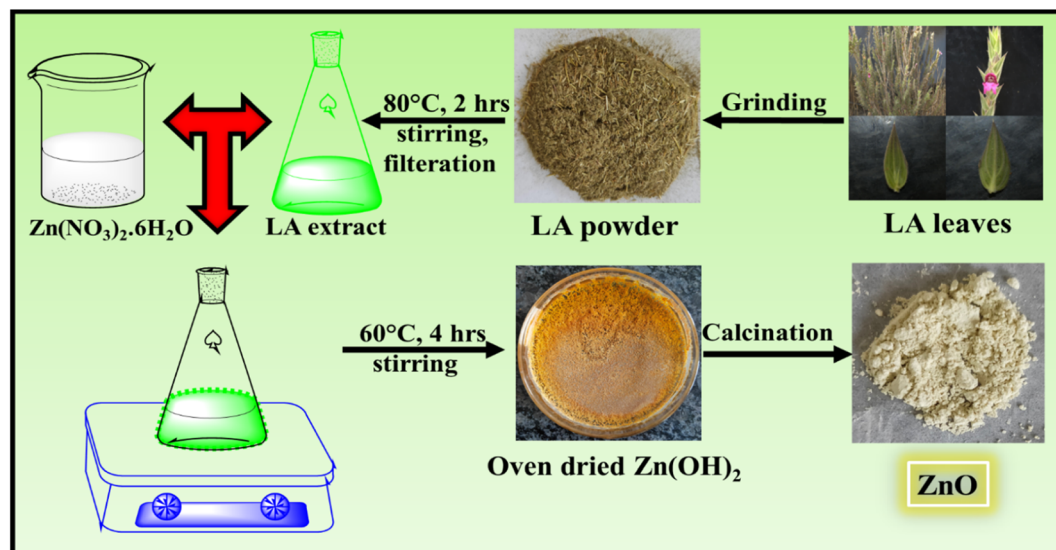
Fig. 1 Schematic representation of synthesis of ZnO NPs using LA leaf template.
