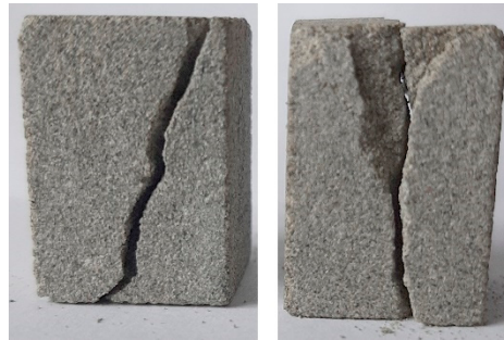
Figure 2. Typical failure patterns of samples.
