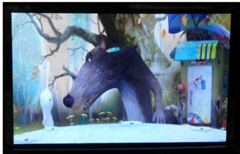
Figure 4. 15-inch blue-phase liquid-crystal display [63]. Invited Paper: The World's First Blue Phase Liquid Crystal Display from Lee, SID Symposium Digest of Technical Papers; published by John Wiley and Sons.
