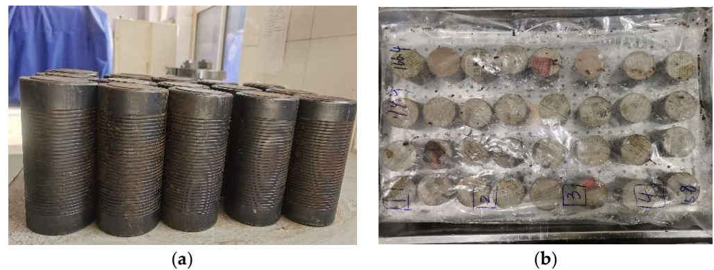
Figure 4. Samples preparation, (a) samples before demolding, (b) samples after demolding.
