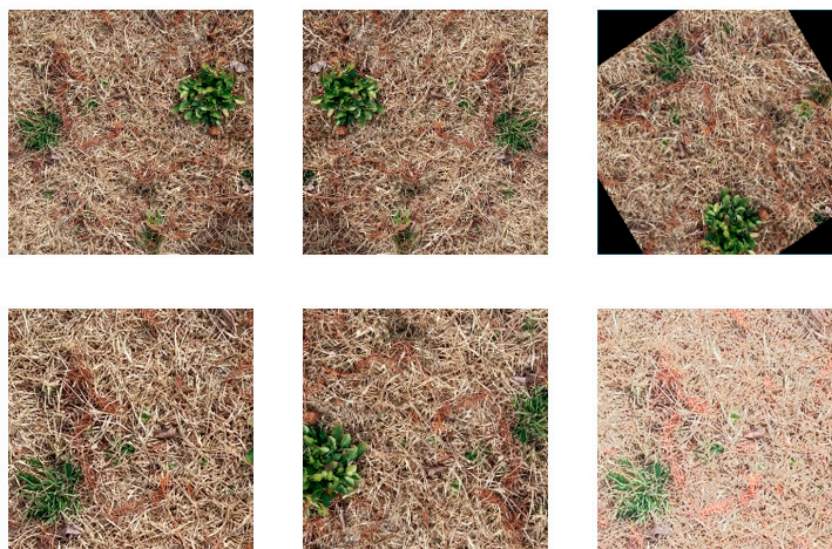
Figure 7. Example images of geometric data augmentation methods (from left to right): original image; horizontal flip; random rotation; random crop; flip + random crop; random crop + photometric distortion.
