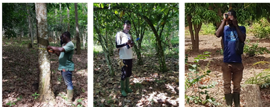
Figure 4. Collection of biophysical parameters of trees in AFS. from left to right: diameter measurement using a diameter tape in a rubber plantation; species identification in a cocoa farm, and height measurement with an altimeter in a mango plantation (field campaign, Côte d'Ivoire, March 2020).
