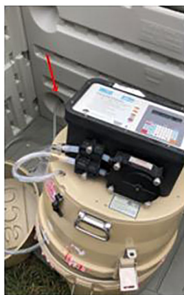
FIGURE 2 Left: Tubing extending outward through the rear of the security box; Center: Tubing coming up the sewer into the security box from beneath manhole cover; Right: Tubing extending directly into manhole opening (one location only)
