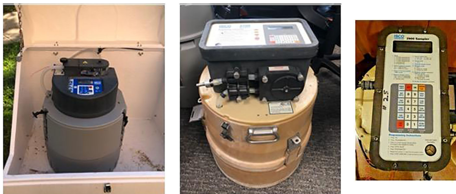
FIGURE 1 Left: ISCO 6712 autosampler as installed in the field. Center: ISCO 3700 being prepped for usage. Right: ISCO 2900 autosampler panel (closeup)
