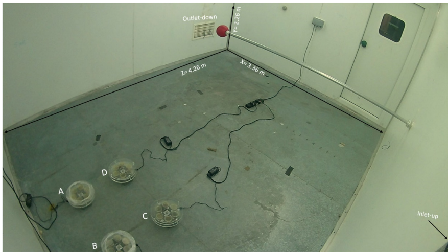
FIGURE 3 Automated multiplate passive air sampling placement in the controlled environment chamber.
