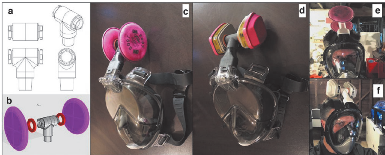
FIG. 4. (a–d) Illustrating varying industrial-grade filters jointed onto the same 3D printed coupler. (e, f) Demonstrate Pneumask being worn.
