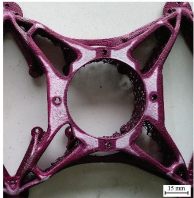
FIG. 2. Result of level 4 dye penetrant test. Color images are available online.
