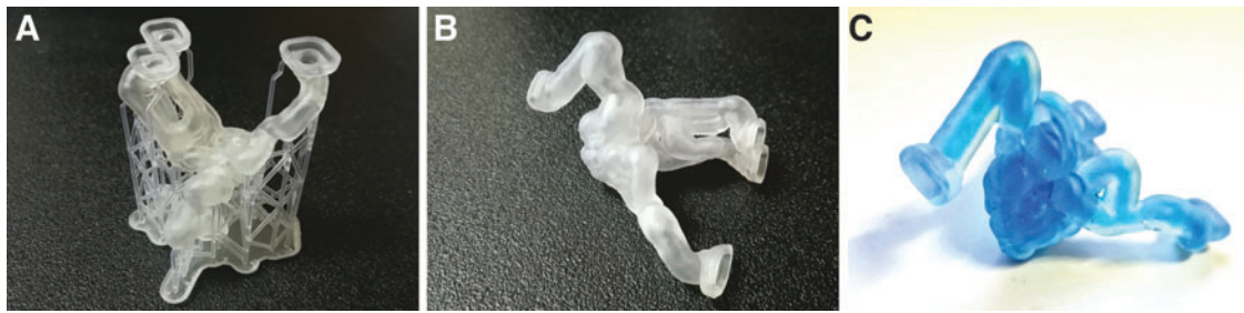
FIG. 3. (A) AVM model straight after printing and (B) after removal of supports. (C) AVM filled with an aqueous solution containing a blue dye. AVM, arteriovenous malformation; CT, computed tomography.
