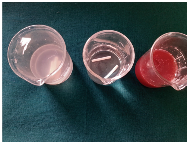
Figure 1: This picture depicts the lime juice, grape juice, and distilled water in which the glass ionomer cement, sample materials has been immersed
