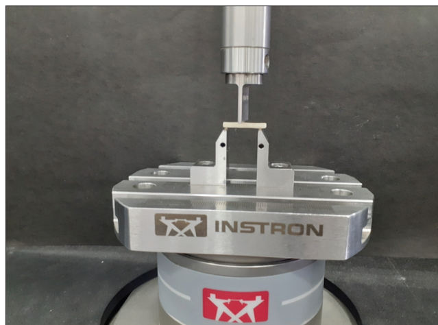
Figure 2: This picture depicts the machine (INSTRON E3000 UTM) used for flexural strength assessment
