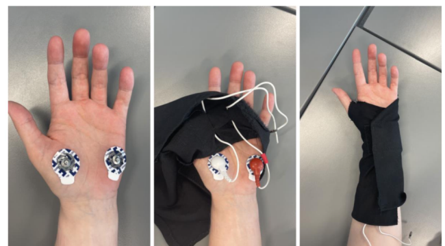
Figure 5: Photo of electrode placement and glove
