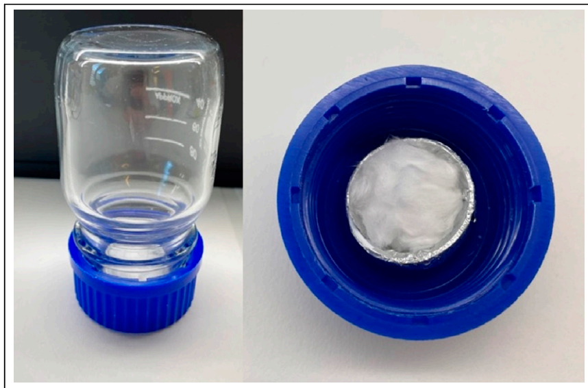
FIGURE 2. Single-chamber ^{212}\text{Pb} generator consisting of glass flask and removable cap that contains ^{228}\text{Th} or ^{224}\text{Ra} source fixed onto porous quartz wool.
