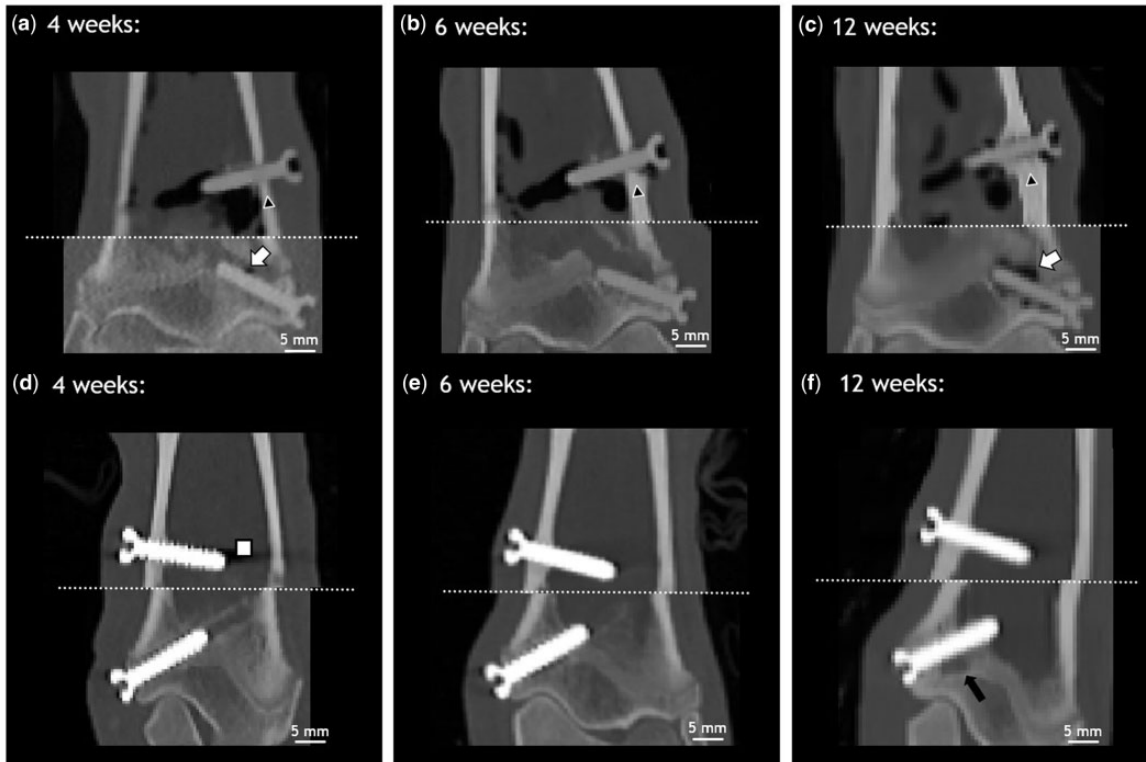
Figure 3. In vivo cCT images of distal tibiae of one animal. ZX00 (a–c) and Ti (d–f) screws 4, 6 and 12 weeks after implantation are shown. White arrows indicate gas formation around the epiphyseal screw (a and c). Cortical thickness increases over time (a–c; black triangle). Some scanning artifacts (white square) were detected around the Ti-screws, mainly at the screw tip 4 weeks after implantation (d). Slight change in trabecular bone structure was detected below Ti-screw after 12 weeks (f; black arrow).
