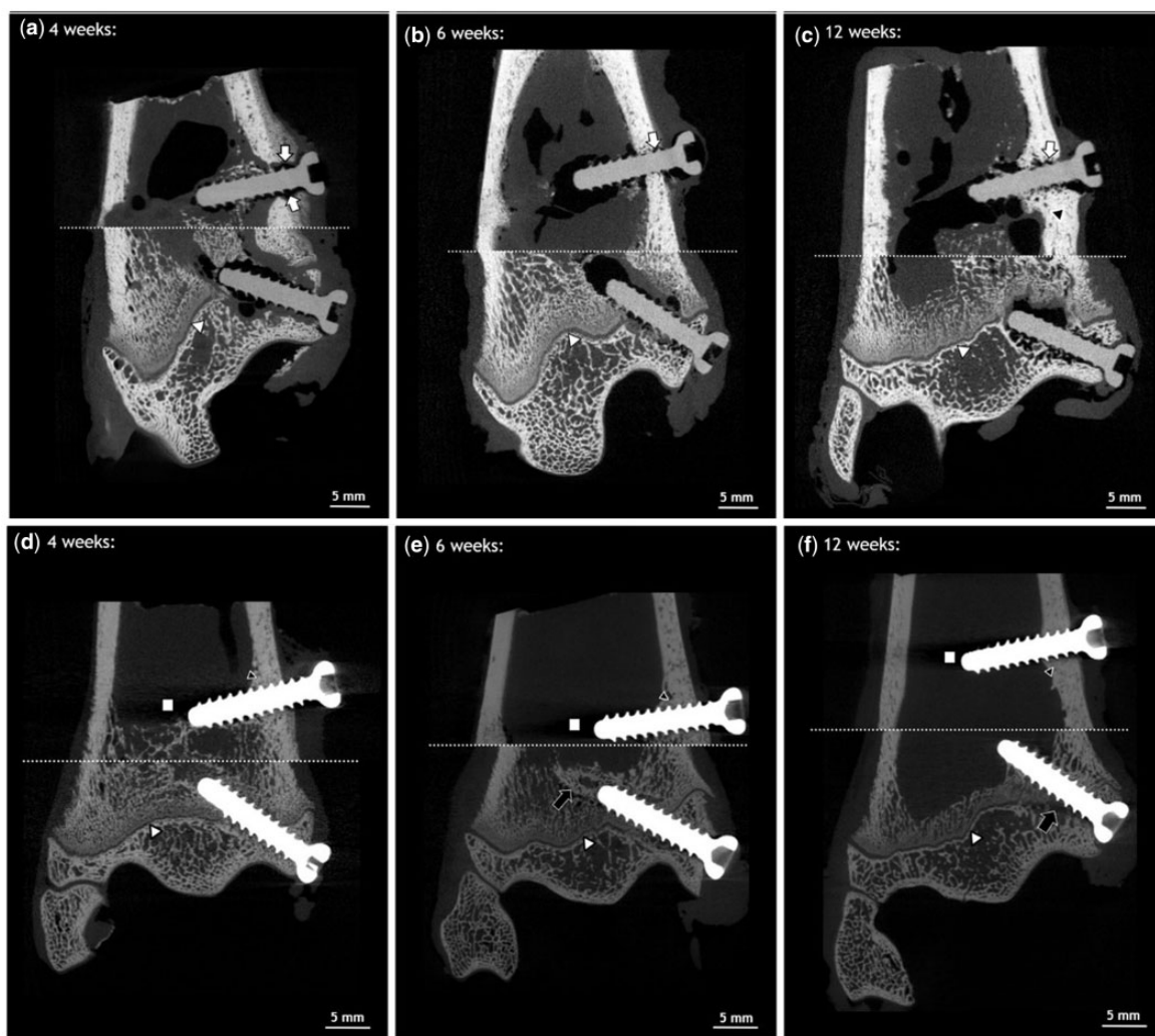
Figure 4. Ex vivo \mu CT images of distal metaphysis and epiphysis. ZX00 (a–c) and Ti (d–f) screws 4, 6 and 12 weeks after implantation. Images of metaphyseal and epiphyseal screws of the same animals were stitched together. The stitching line is marked with a white dotted line. Increased cortical thickness was detected around ZX00-screw after 12 weeks (black triangle). Small gas pockets were found in the cortical bone around the ZX00-screw after 4, 6 and 12 weeks (white arrows). Slight alterations in trabecular bone structure around Ti-screws were detected 6 and 12 weeks after implantation (e and f; black arrows). Scanning artifacts were found only around Ti-implants (d–f; white squares). The physis was detected in all animals (a–f; white triangle), interrupted by the implant.
