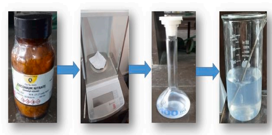
Fig. 2. Steps of making the aqueous solution of ZrO(NO_3)_2 .
