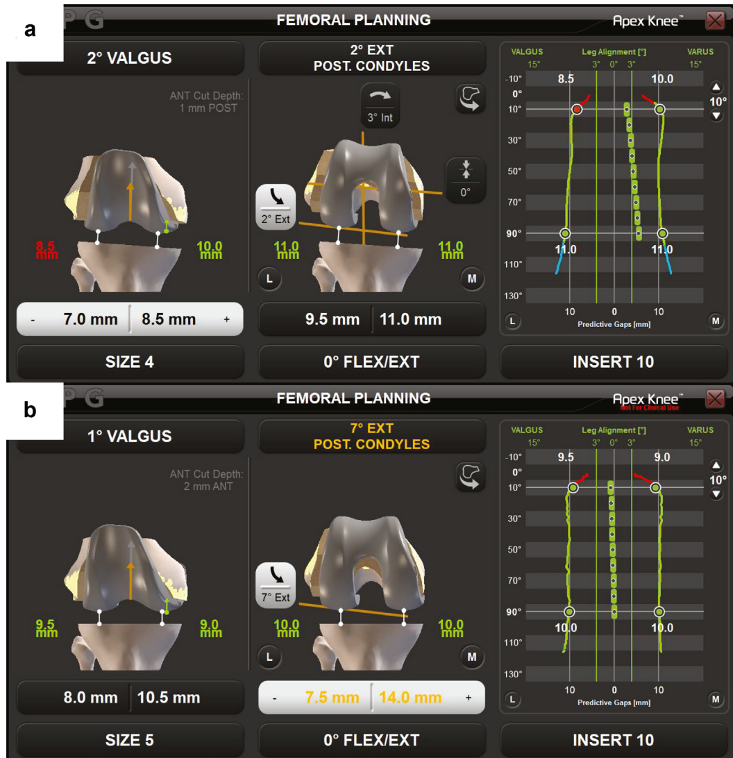
Figure 2. Femoral planning screen for piKA (a) and pGB (b). Femoral component position can be adjusted with the computer navigation system intraoperatively. The predictive soft tissue laxity plan is then visualized throughout the flexion range.
