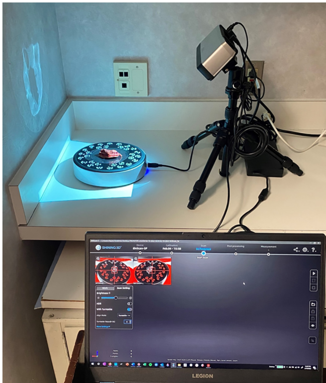
Fig. 1. Structured light 3D scanning setup used for image acquisition in our lab. The specimen is placed in the center of the scanner turntable on a translucent plastic sheet. The computer (bottom right) demonstrates the software used to capture the surface topography of the specimen.
