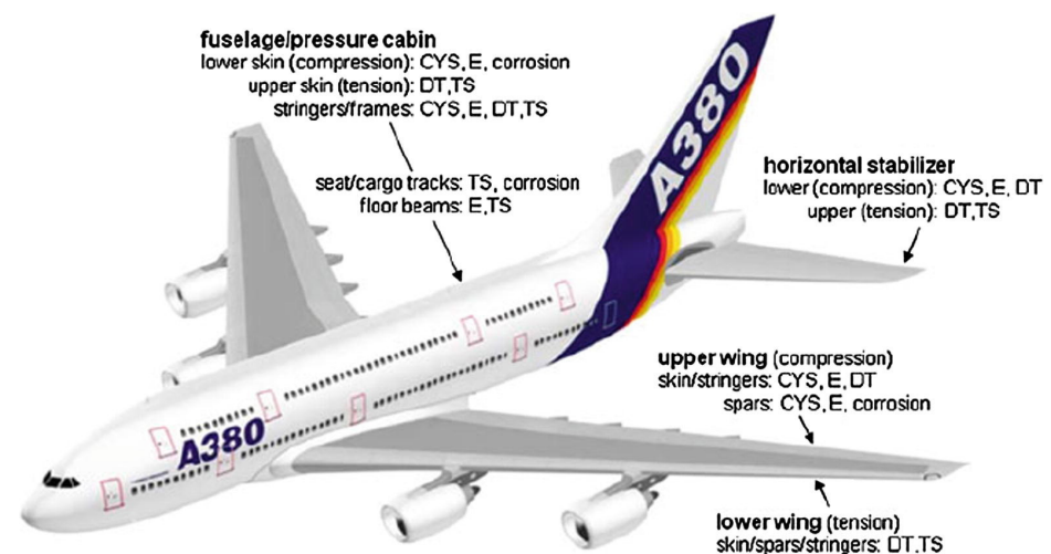
Figure 3. The application of Al alloys in aircraft. Reprinted from Ref. [10] with permission. Copyright 2018, Elsevier.
