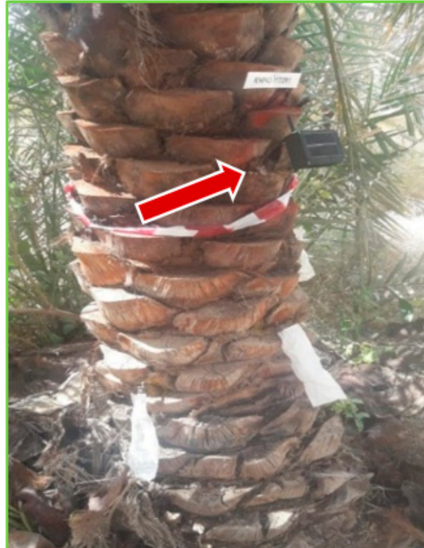
Figure 3. The installed acoustic sensor on a date palm trunk. The arrow is showing the device probe inserted inside the date palm tree trunk.
