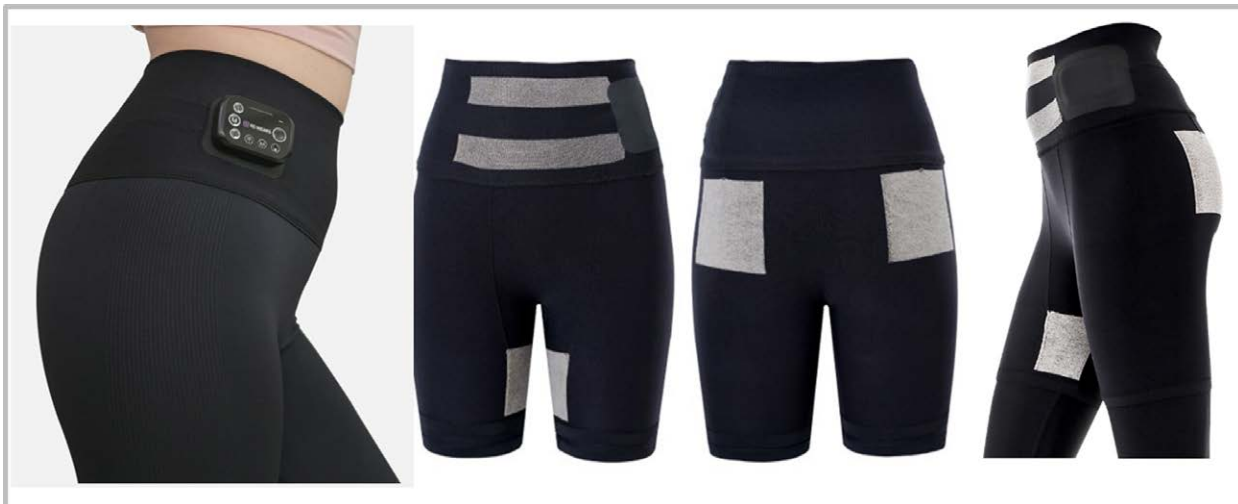
Figure 2. The wearable EMS training pants and positioning of the electrodes. EMS = electrical muscle stimulation.
