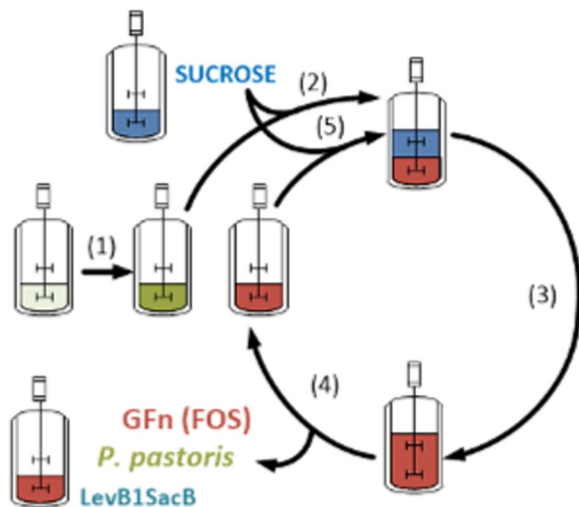
Fig. 1 Layout of the simultaneous enzyme production, enzymatic reaction, and glucose elimination fermentation system. (1) Glucose induced Enzyme production (EP) stage; (2) First enzyme production (EP) and enzyme reaction (ER) stages; (3,4,5) Productive fed batch (FB) stages: the enzyme is now induced by residual glucose from the reaction. Half of the culture is retired after each batch and replenished with fresh culture medium containing sucrose. See text for a detailed description
