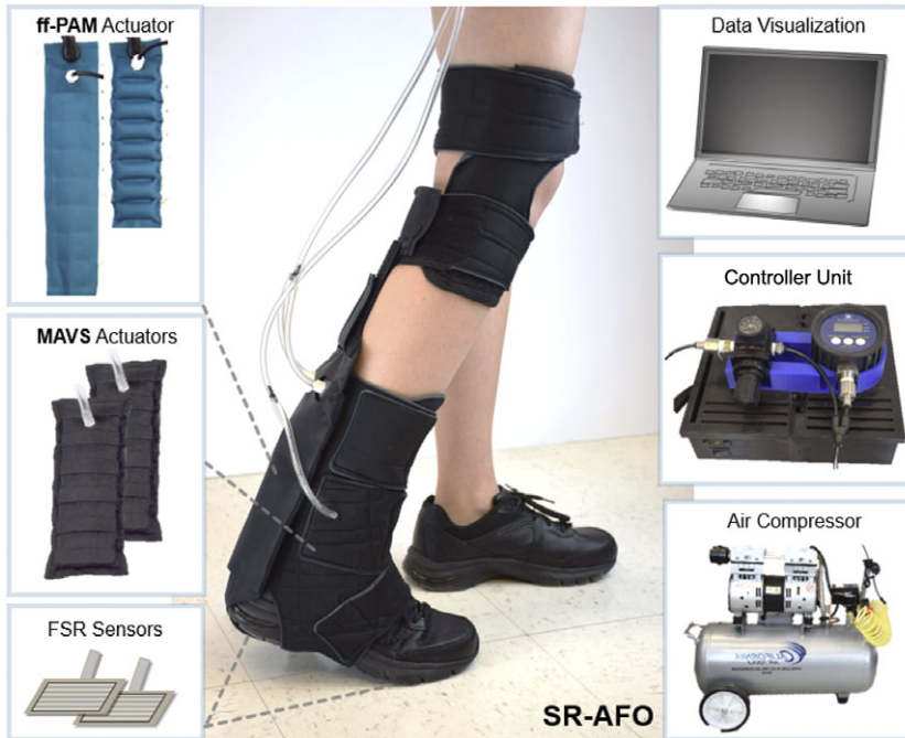
Figure 11. (Middle) The final assembly of the soft robotic ankle-foot orthosis and its components. (Left) The flat fabric pneumatic artificial muscle and multi-material actuator for variable stiffness actuators and the force-sensitive resistor sensors for gait detection. (Right) The controller, pneumatic source (air compressor), and visual feedback for system operation.
