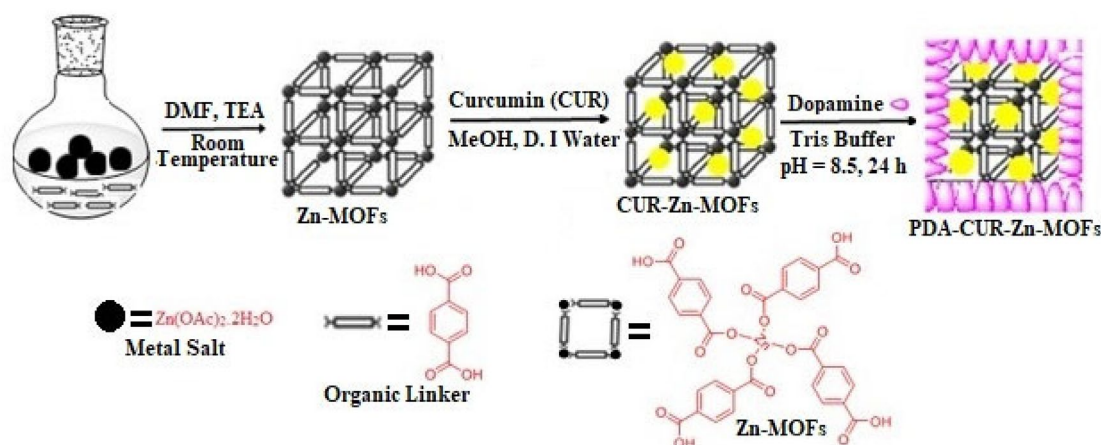
Scheme 1. Synthesis routes for the preparation of PDA-CUR-Zn-MOFs.
