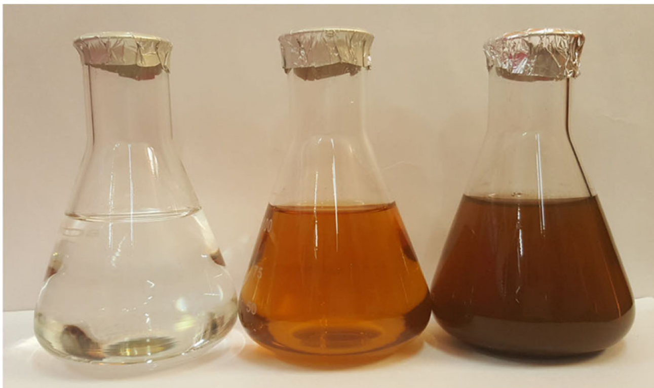
Fig. 5 A comparison of the colour intensity of the aqueous extract of Malva sylvestris before and after reducing the amount of silver nitrate (1 mM). The change in hue shows that Ag + has been reduced to an elemental nanosilver (Govindarajan et al. 2016)
