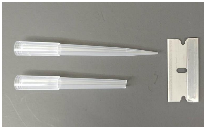
Figure 4. Preparing pipette tips for viscous solutions. Comparison of an uncut 1,000 \mu L pipette tip (top) and a tip with approximately 2 cm cut off with a razorblade (bottom).
