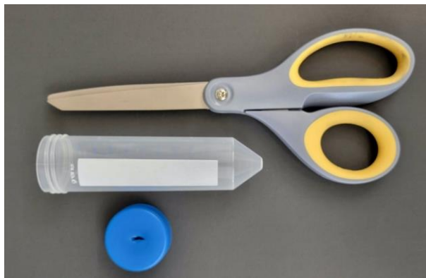
Figure 7. Preparing a 50 mL conical tube for frozen yeast pellets. Photo of a 50 mL conical tube and punctured lid to store frozen yeast pellets. The punctured lid allows liquid nitrogen to vent after cell pellets have been poured into the tube.
