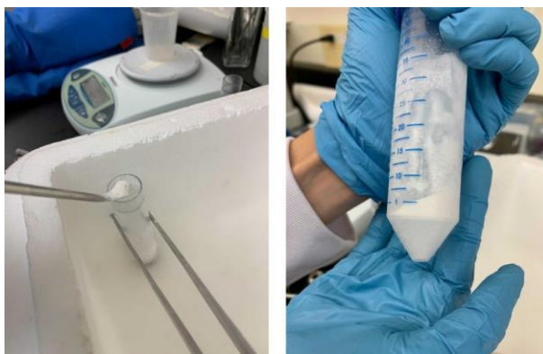
Figure 10. Handling yeast powder. (Left) Photo showing the loose and fluffy consistency of the lysed yeast powder when handled and stored at -80^{\circ}\text{C} or colder. (Right) Example 2 g aliquot of yeast powder stored in a 50 mL conical vial.
