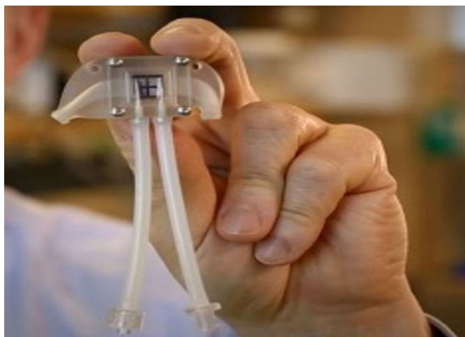
Figure 4. A prototype of the implantable bioartificial kidney.
