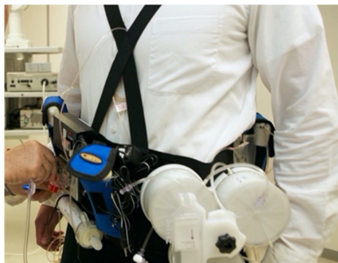
Figure 1. Prototype of the wearable artificial kidney. Filtration components are attached to a belt for the patient to wear.
