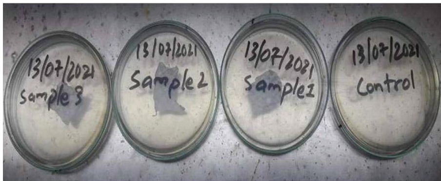
FIGURE 6: The contamination test of DFS scaffold. The test was performed on three identical DFS scaffolds, and there was no bacterial growth on the sample.
