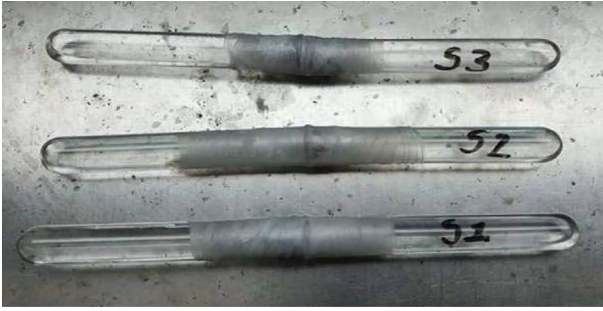
FIGURE 10: The permeability test of the DFS scaffold of different samples.
