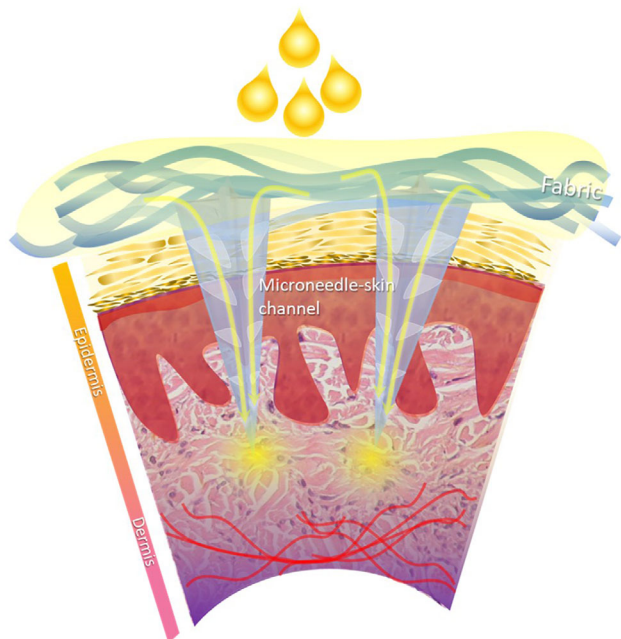
FIGURE 2 The active ingredient or solution delivery mechanism of the four-point star-shaped microneedle array fabricated on the fabric substrate
