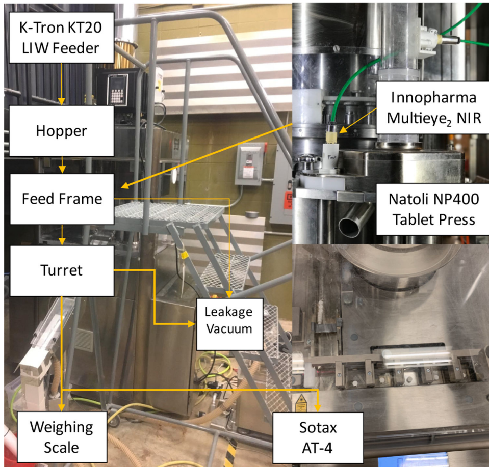
Fig. 6. A photo of a subset of the OSD-CM process to illustrate CBM systems architecture.
