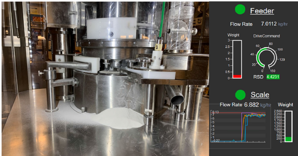
Fig. 15. Leakage arising from wear in the tablet press, with usage of mass balance for condition monitoring.
