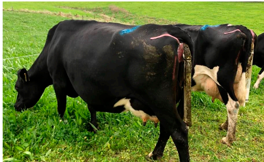
Figure 1. PEETER V1.0 urine sensors attached to cows during the experiment.
