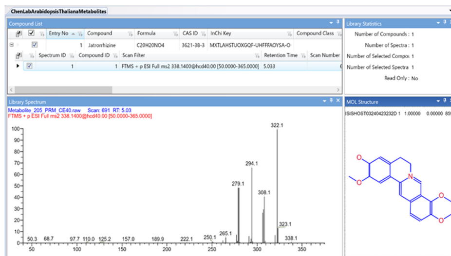
Figure 2. Full MS spectra and MS/MS spectra of metabolite 205 (jatrorrhizine) acquired at different normalized collision energy (NCE) values. (a) Full MS of jatrorrhizine. Top panel, experimental data; bottom panel, theoretical isotopic pattern. (b) MS/MS spectra of jatrorrhizine. The fragmentation spectra were acquired at NCEs of 20, 30, 40, and 50 eV from the top to bottom. (c) Entry of the jatrorrhizine spectra into the mzVault library (showing NCE 40 eV spectrum as an example).
