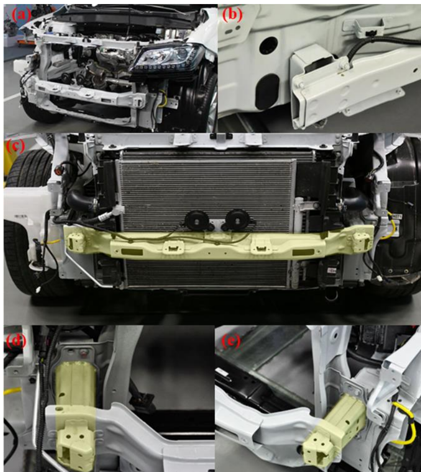
Figure 2. Steel bumper beam and crash box of Haval H2. (a) Front frame, (b) rear bumper beam, (c) front bumper beam and steel buffer plate, (d) left crash box, (e) right crash box.
