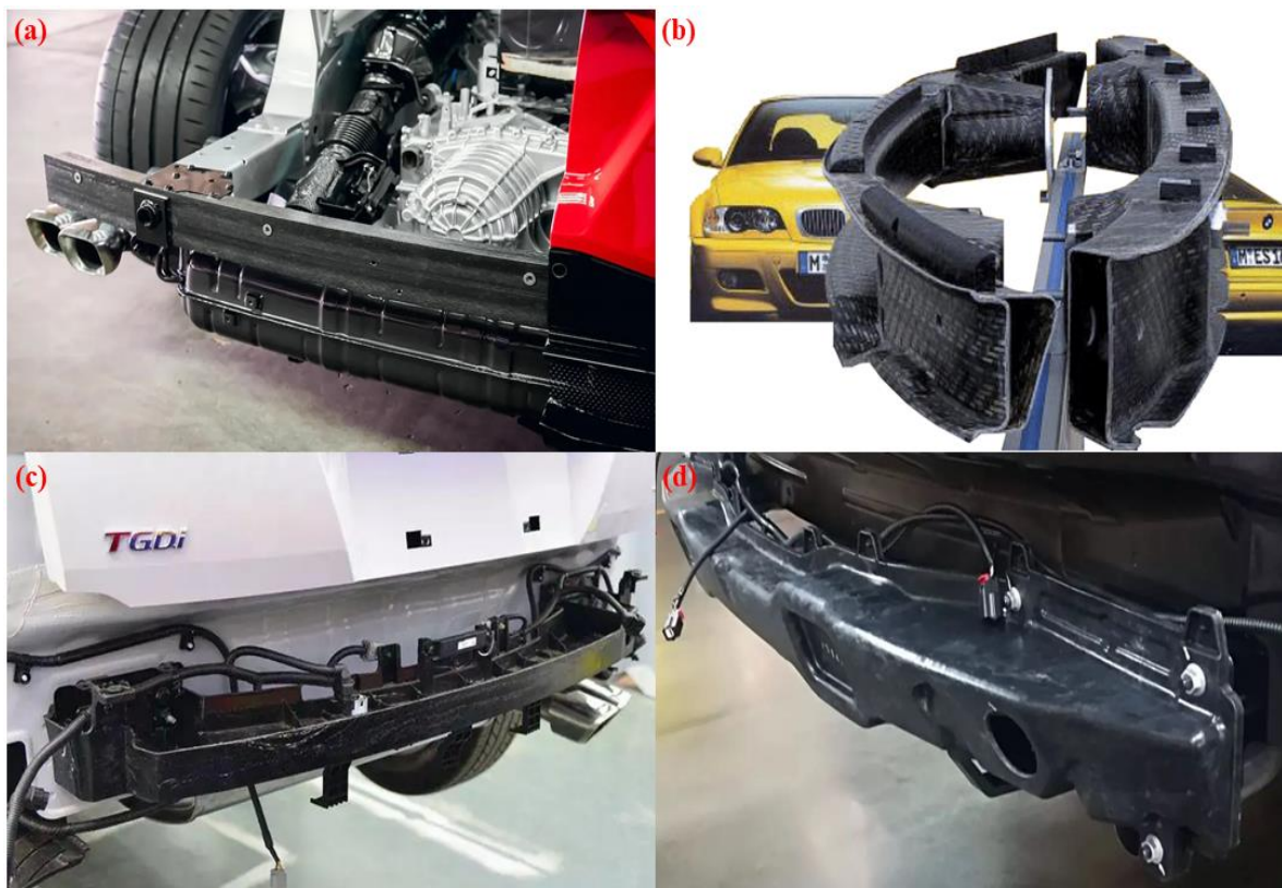
Figure 3. Application of composites in bumper beam. (a) Corvette C8, (b) BMW M3, (c) Hyundai TUCSON, (d) GEELY Emgrand X7 Sport.
