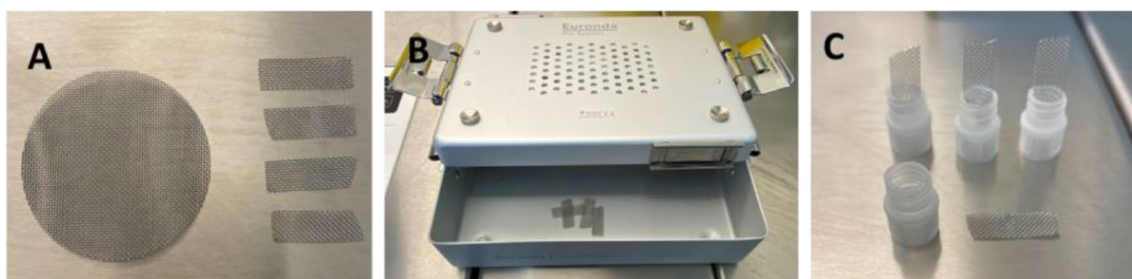
Fig. 2 Preparation of material. Metal cell meshes were cut to 25 \times 8 mm stripes (A) and prepared for autoclaving (B). After sterilization, meshes were linked with caps of 1.8 ml vials (C) under sterile air conditions
