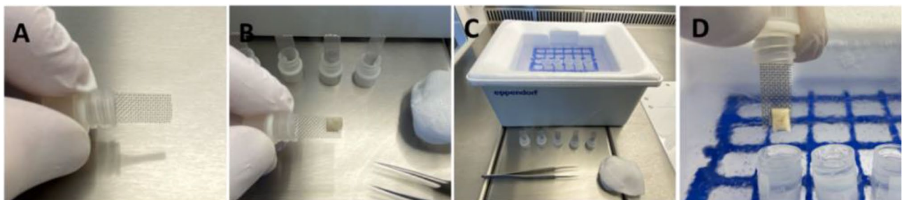
Fig. 4 High-throughput vitrification of ovarian tissue. Ovarian cortex tissue placed on a loading device (A, B) for rapid vertical vitrification (D) in a vial based closed system on a customized, grid based styrofoam device (C), capable of high sample throughput
