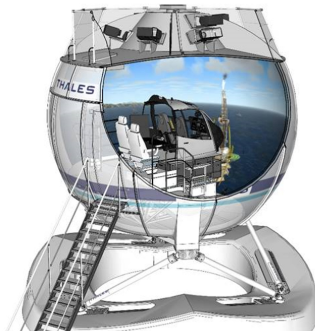
FIGURE 1 The EC135 cabin is in the display dome and the dome is over the six-degrees-of-freedom motion platform. The pilot is seated in the cabin.
