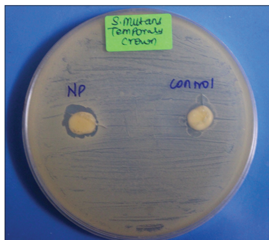
Figure 2: Zone of inhibition seen against Streptococcus mutans in the sample modified by chitosan nanoparticles
