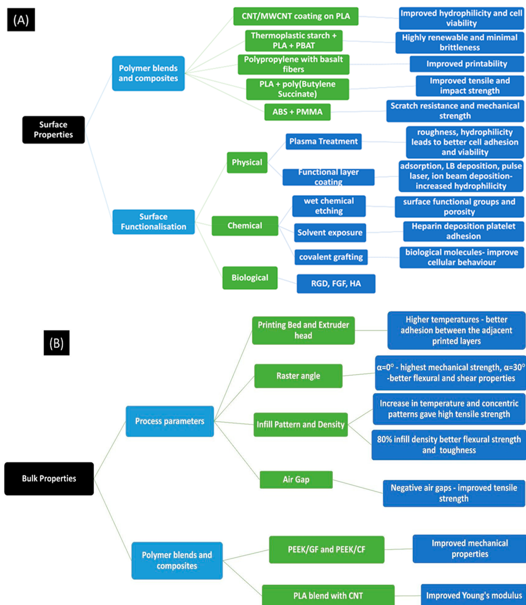
Figure 9. (A, B) Summary of surface and bulk parameters improved for tissue engineering applications through changes in process parameters and 3D-printer properties.
