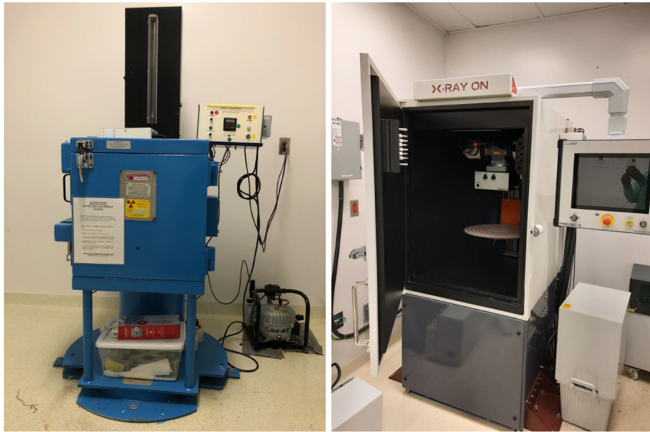
Figure 1. Irradiators used in our experiment: Mark I-68 ^{137}\text{Cs} irradiator (left) and X-Rad320 x-ray irradiator (right).
